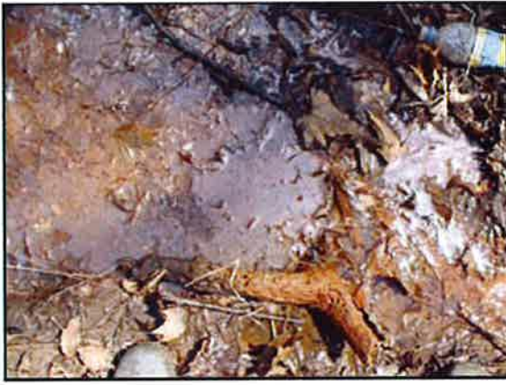
Figure 8.4.6: Synthetic versus Natural Sheen (a) Sheen from bacteria such as iron floc forms a sheet-like film that cracks if disturbed (b) Synthetic oil forms a swirling pattern
