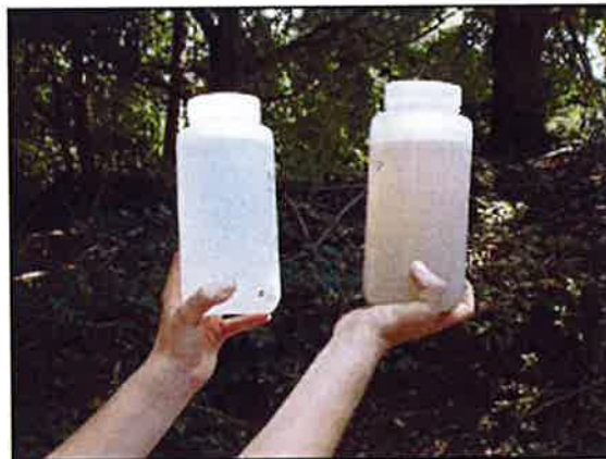
Figure 8.4.3: Using a sample bottle to estimate color and turbidity
