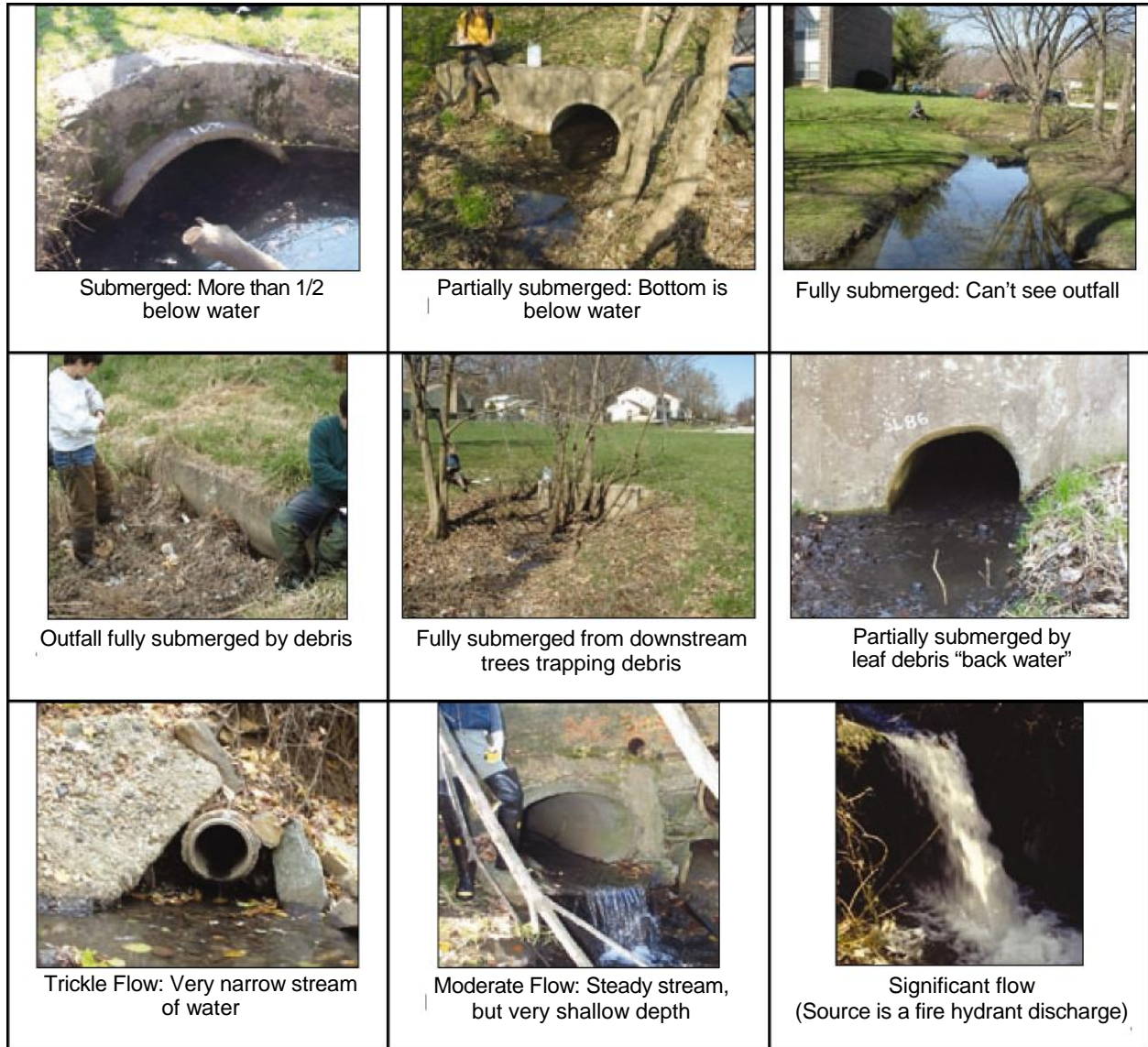
Figure 8.4.1: Characterizing Submersion and Flow
