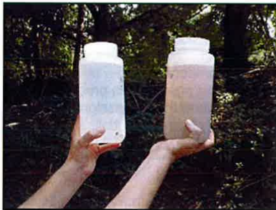
Figure 8.4.3: Using a sample bottle to estimate color and turbidity
