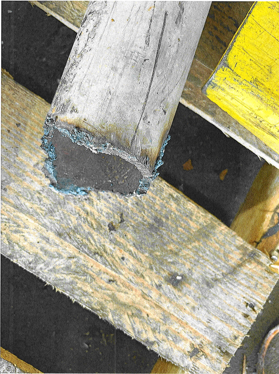
Upper oil tube. This is where I had to use the plasma cutter to cut through the stainless steel to release the stuffing box. Oil tube and stuffing box would not unthread from each other. Will need a new oil tube.
